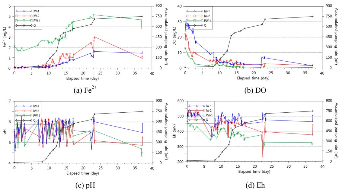
Fig. 6. Changes in  $\text{Fe}^{2+}$ , DO, pH, and Eh after stopping a continuous injection of oxygenated water. (a)  $\text{Fe}^{2+}$ , (b) DO, (c) pH, (d) Eh.
