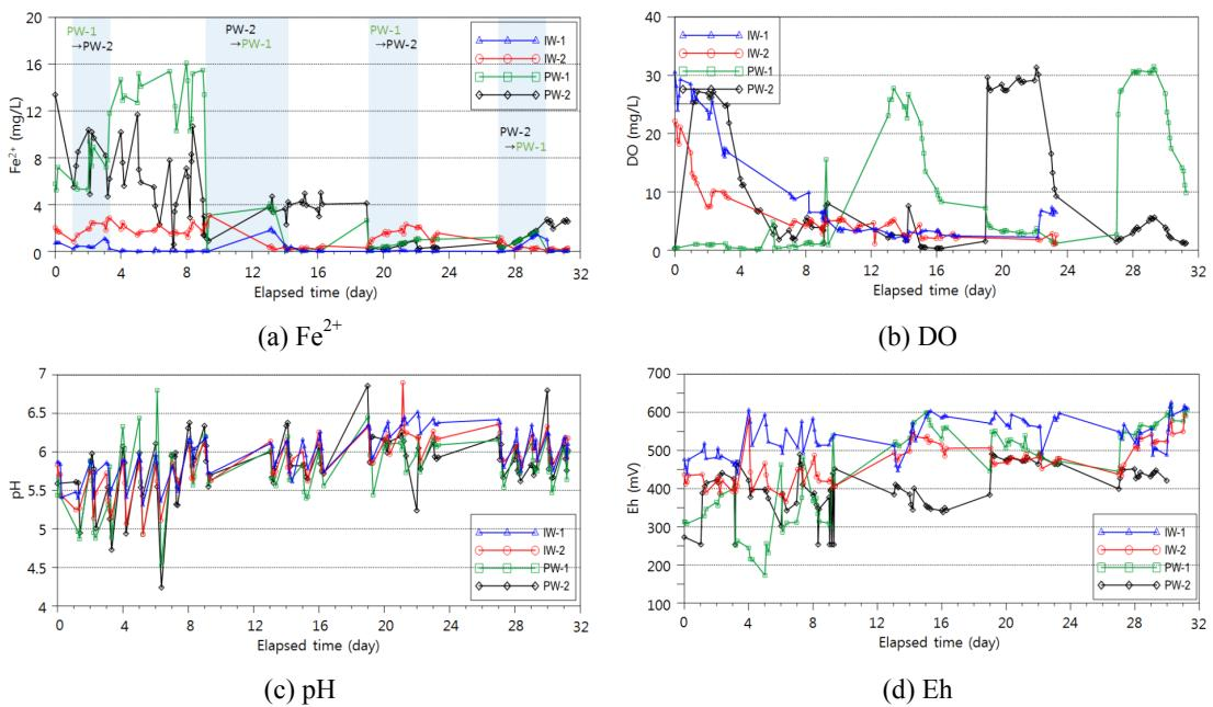
Fig. 7. Changes in  $\text{Fe}^{2+}$ , DO, pH, and Eh during an alternating injection of oxygenated water. (a)  $\text{Fe}^{2+}$ , (b) DO, (c) pH, (d) Eh.
