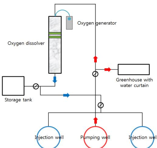
**Fig. 3.** In situ iron treatment system using an injection process of oxygenated water.
