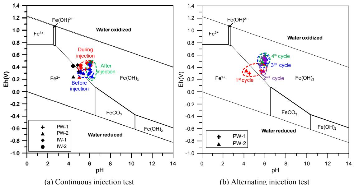
Fig. 8. pH-Eh diagrams of the  $\text{Fe}-\text{CO}_2-\text{H}_2\text{O}$  system under two test conditions:  $\text{Fe}_T = 10^{-4} \text{ M}$  and  $C_T = [\text{H}_2\text{CO}_3] + [\text{HCO}_3^-] + [\text{CO}_3^{2-}] = 10^{-2.5} \text{ M}$ . (a) Continuous injection test, (b) Alternating injection test.
