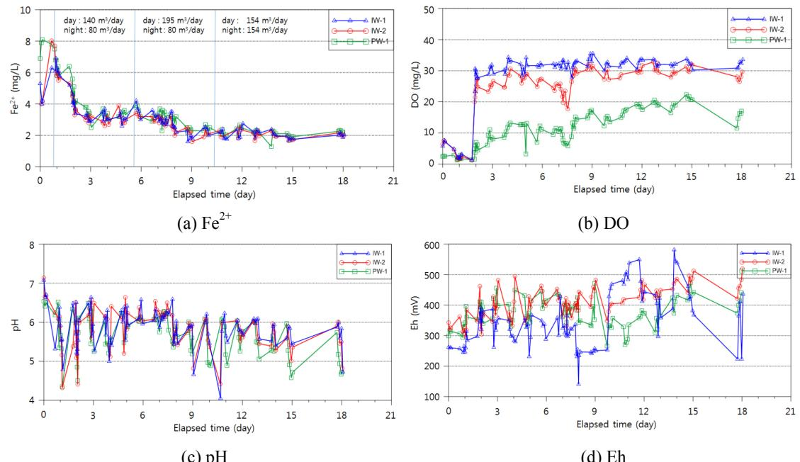
**Fig. 5.** Changes in  $\text{Fe}^{2+}$ , DO, pH, and Eh during a continuous injection of oxygenated water. (a)  $\text{Fe}^{2+}$ , (b) DO, (c) pH, (d) Eh.
