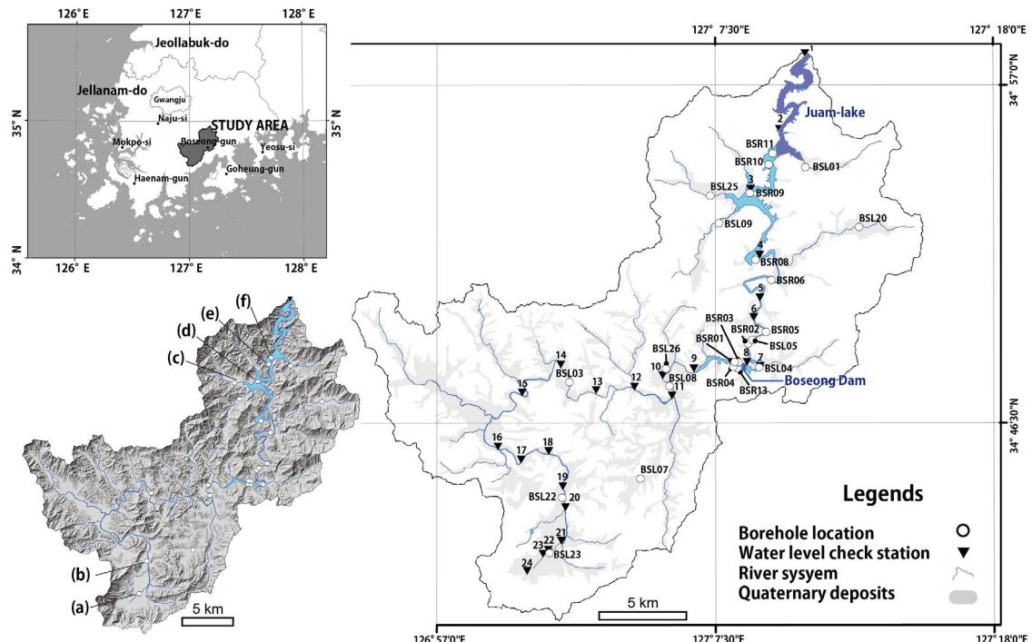
**Fig. 1.** Borehole locations and water-level check stations in the study area. a ~ f show the locations of overview photo in Fig. 2.
