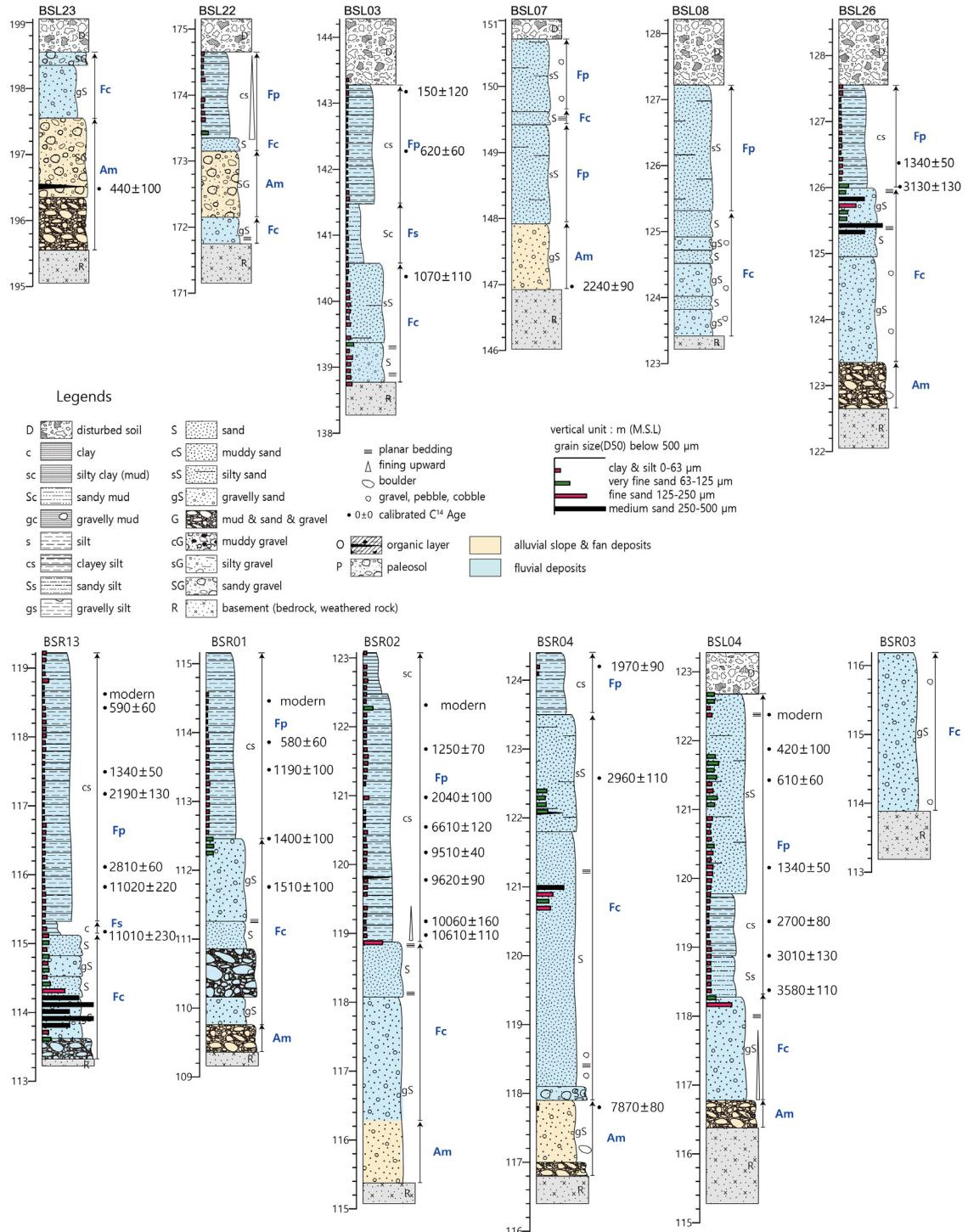
**Fig. 4.** Stratigraphy of the boreholes with simplified lithology, depositional environments, facies types and calibrated radiocarbon dating ages. Note the elevation is meter scale from GPS survey.
