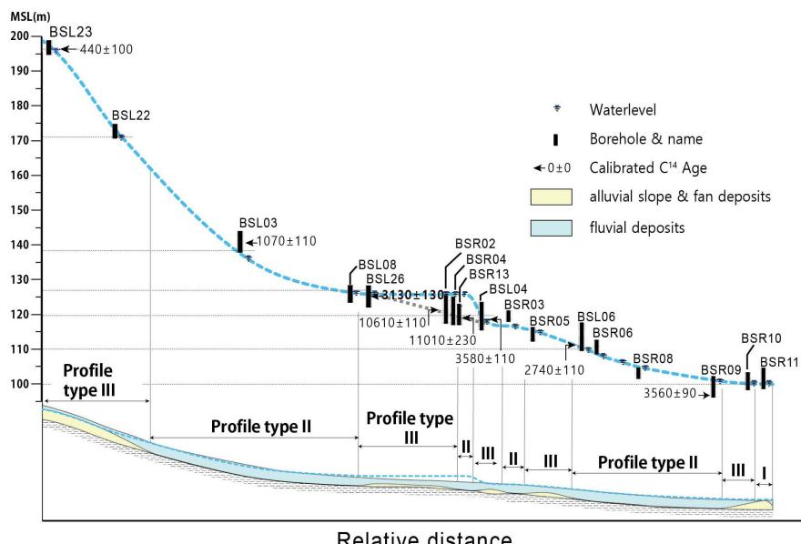
Fig. 5. Schematic diagram of profile types inferred from stratigraphic column of the Quaternary sediments.
