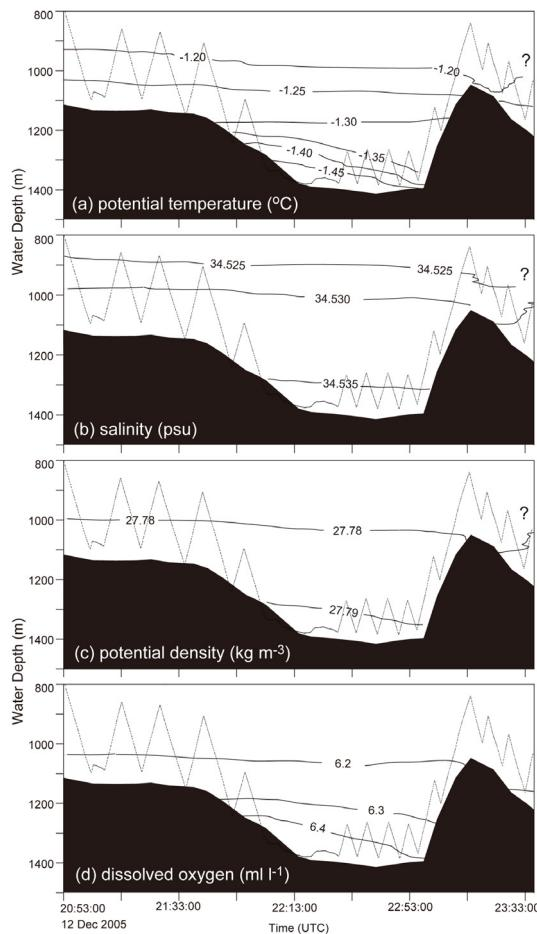
**Fig. 8.** Water column characteristics of CTD towing in C'-C line. (a) Potential temperature ( $^{\circ}$ C), (b) salinity (psu), (c) potential density ( $\text{kg m}^{-3}$ ) and (d) dissolved oxygen ( $\text{ml l}^{-1}$ ). The dotted line indicates actual 27.78 isopycnal.
