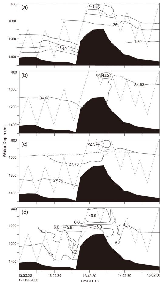
**Fig. 6.** Water column characteristics of CTD towing in A'-A line. (a) Potential temperature ( $^{\circ}\text{C}$ ), (b) salinity (psu), (c) potential density ( $\text{kg m}^{-3}$ ) and (d) dissolved oxygen ( $\text{ml l}^{-1}$ ). The dotted line indicates actual 27.78 isopycnal.
