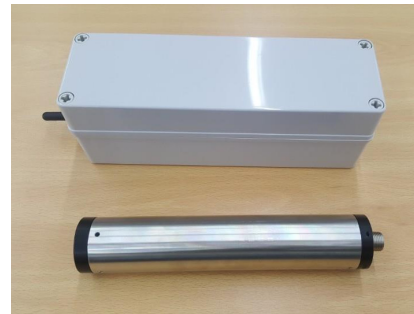
(c) Radon-beta emission monitoring sensor and data logger
