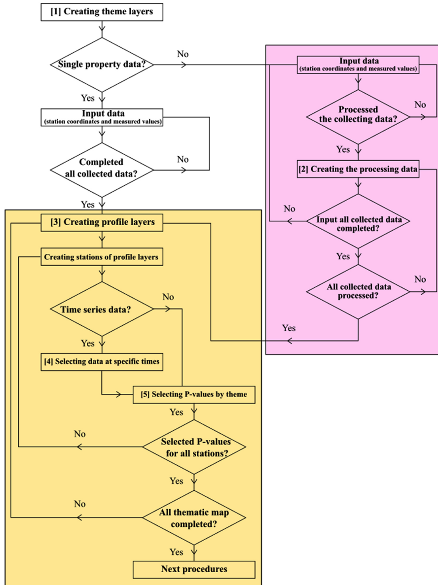
Fig. 2. Procedures for creating theme layers of geological information (The pink-colored area is related to the domain transformation of multi-property data while the yellow-colored area to the creation of theme layers and the choice of P-value from the collected or the processed data produced from the pink-colored area).
