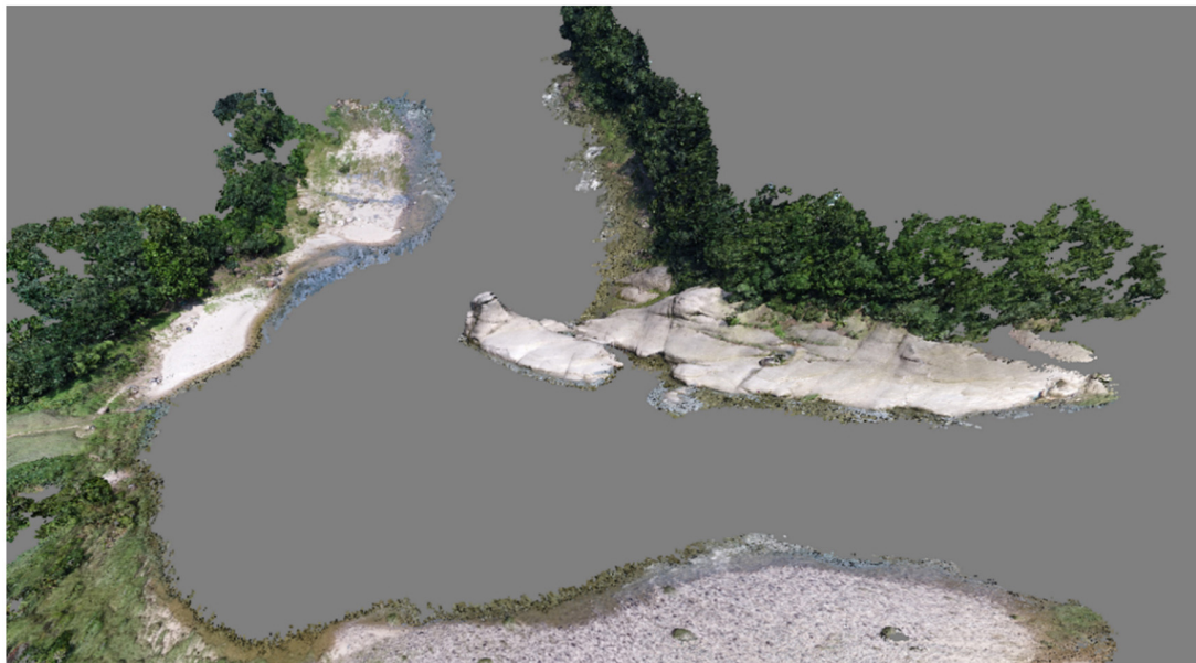
(a) Dense Point cloud by SfM Algorithm
