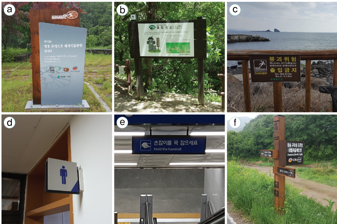
Fig. 1. Different and basic types of guide signs. (a) stand type, (b) pillar type, (c) bond type, (d) protrusion type, (e) ceiling hanger type, (f) wing type.
