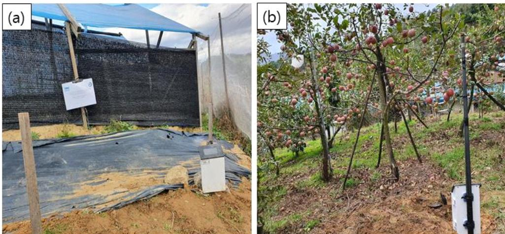
Fig. 3. (a) Ginseng field and (b) apple orchard with automatic soil moisture content monitoring system.
