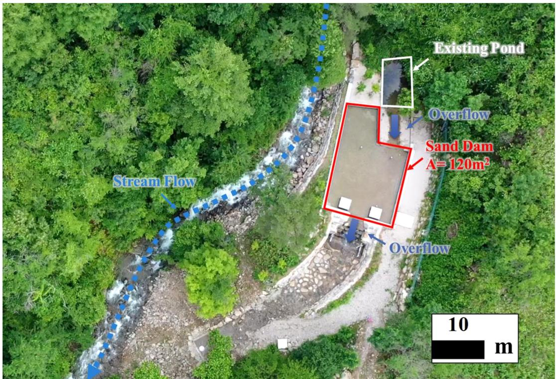
Fig. 1. Location of hydrological component around the sand dam and their area.
