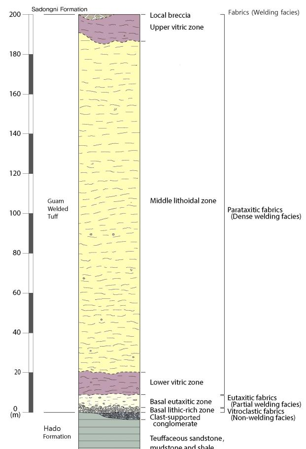
**Fig. 2.** Schematic generalized columnar section of the Guam Welded Tuff, demonstrating field relationships and the internal textures in a representative portion from the Hado village to the Yujusan mount: the lithological zones and textures depicted are only examples of features highlighted in other figures.
